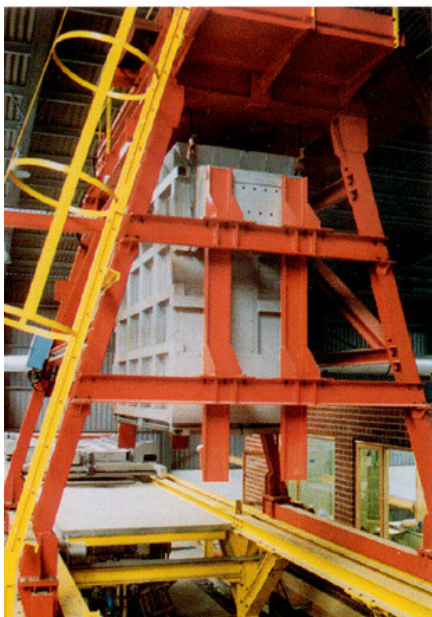
◀ Bomb door type charger and bin (capacity 8000 kg)
