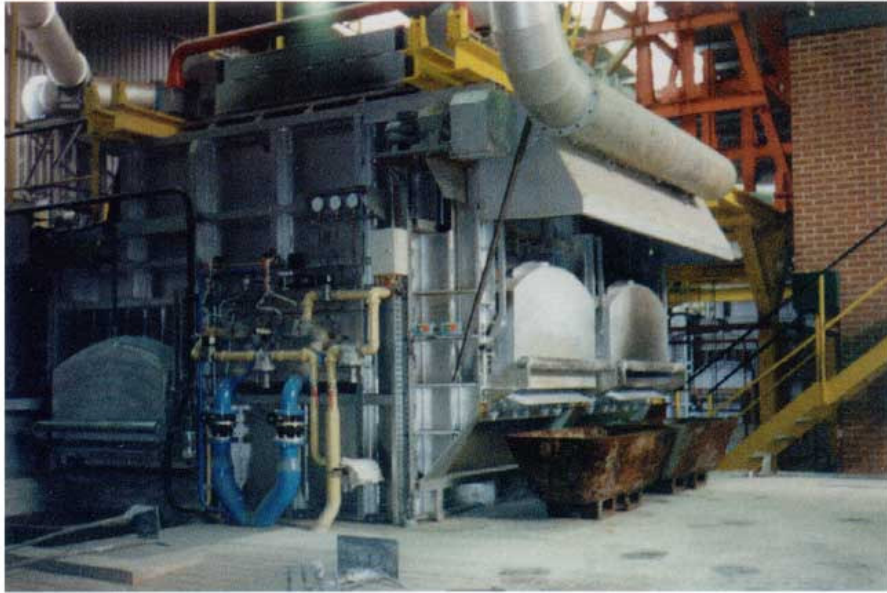
▲ Melting furnace TT 4000 FSAI with combined 30 tonne holding well
