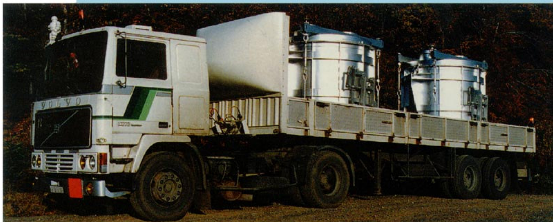
▲ Road transport of molten aluminium
